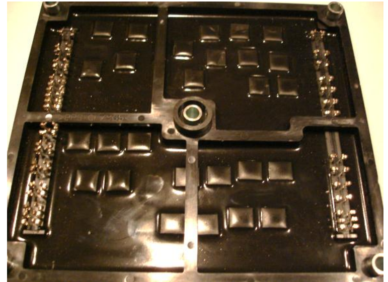
Electronics module (includes rectifiers, inverters)
